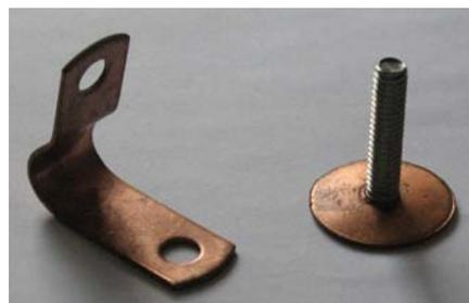
terminals can be soldered directly to copper roof or flashing elements as shown in Figure 1 (see reverse) to eliminate penetrations associated with mechanical fasteners. Any soldering associated with the attachment hardware should be performed by the roofing contractor.
