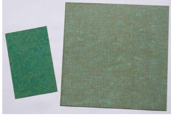
Samples of pre-patinated copper products: SMC-Oxidized Copper Patina 3000 by Unimet Metal Supply (left) and Evergreen® by Revere Copper (right).
